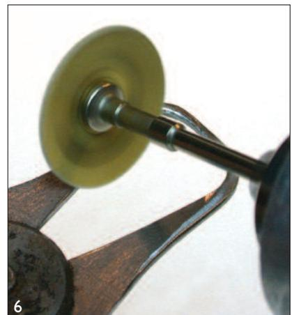
a light touch, round the corners of the tips of the jaws on both gauges. Be sure to leave the points rounded, and don't remove material from the very center of the jaws or you'll have to adjust them back to zero (7).
